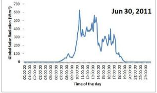
Figure 12: Diurnal plot of Global Solar Radiation for June 30, 2011
